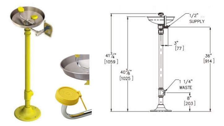
Model S0340 is our free standing eye wash with stainless steel bowl. Comes complete with stainless steel bowl, plastic eye/face wash spray heads, an inline strainer and a stay-open 1/2" ball valve with a push handle. Pedestal mounted to allow freedom of being positioned away from walls.
